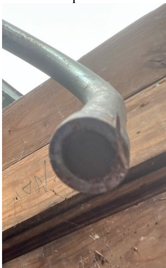
S01 well vent screen intact.
