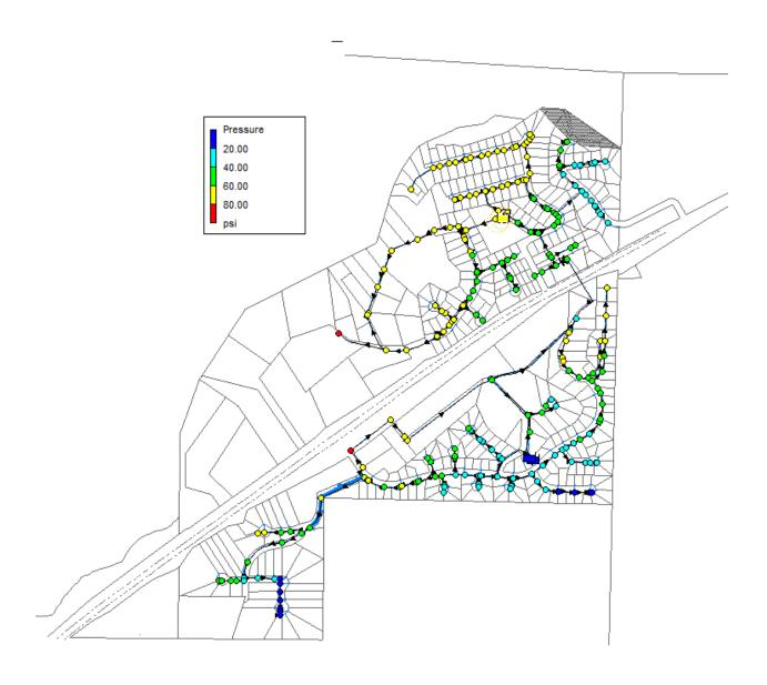
Figure 1 – Scenario 1: Multiplier of 1.8 gpm/node, full build-out
