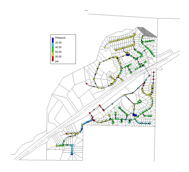
Figure 3 – Scenario 3: Multiplier 1.05 gpm/node, pressure at all connections >20 psi
