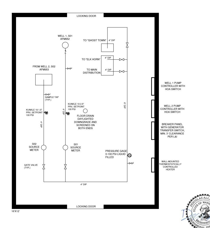
PROPER VENTING, INSULATION AND PANELING, WALL MOUNTED THERMOSTATICALLY CONTROLLED HEATER, LIGHTING, GFI OUTLET, L. AND I. APPROVED WIRING, AND RODENT PROOF
